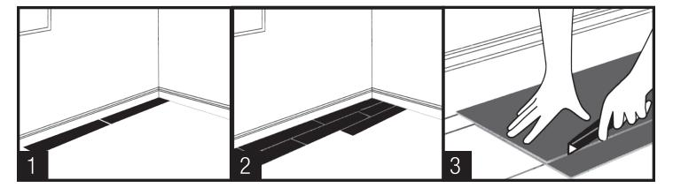
by the adhesive manufacturer. Avoid spreading more adhesive than needed, as the adhesive will lose its ability to fully stick to the back of the planks.
